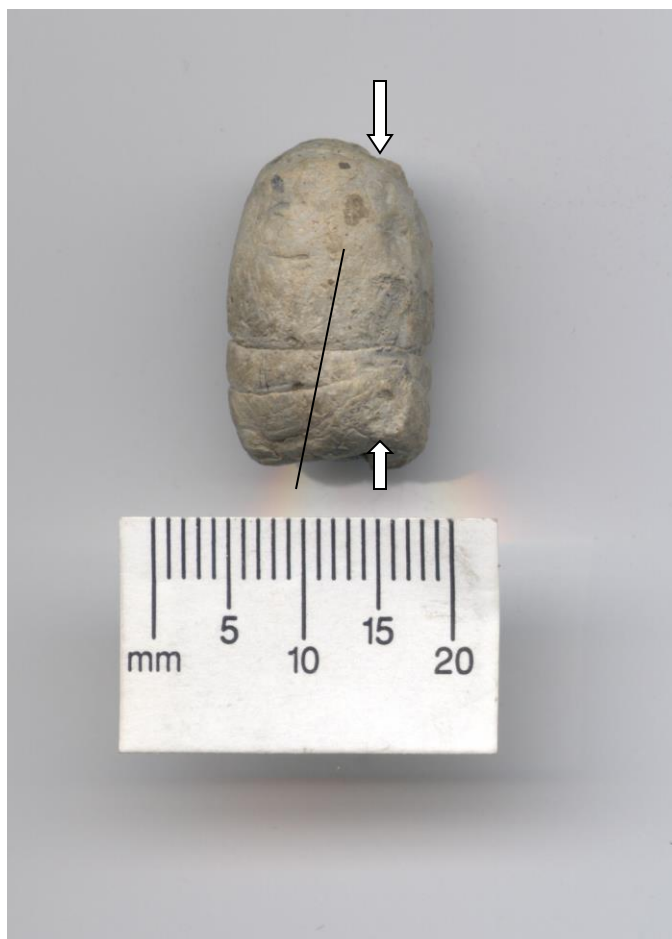
Figure 2. The bullet highlighted to show various diagnostic features and impact damage: top arrow points to nose damaged area, bottom arrow points to base damage, and the line denotes the right-hand twist of the land and groove impression.
